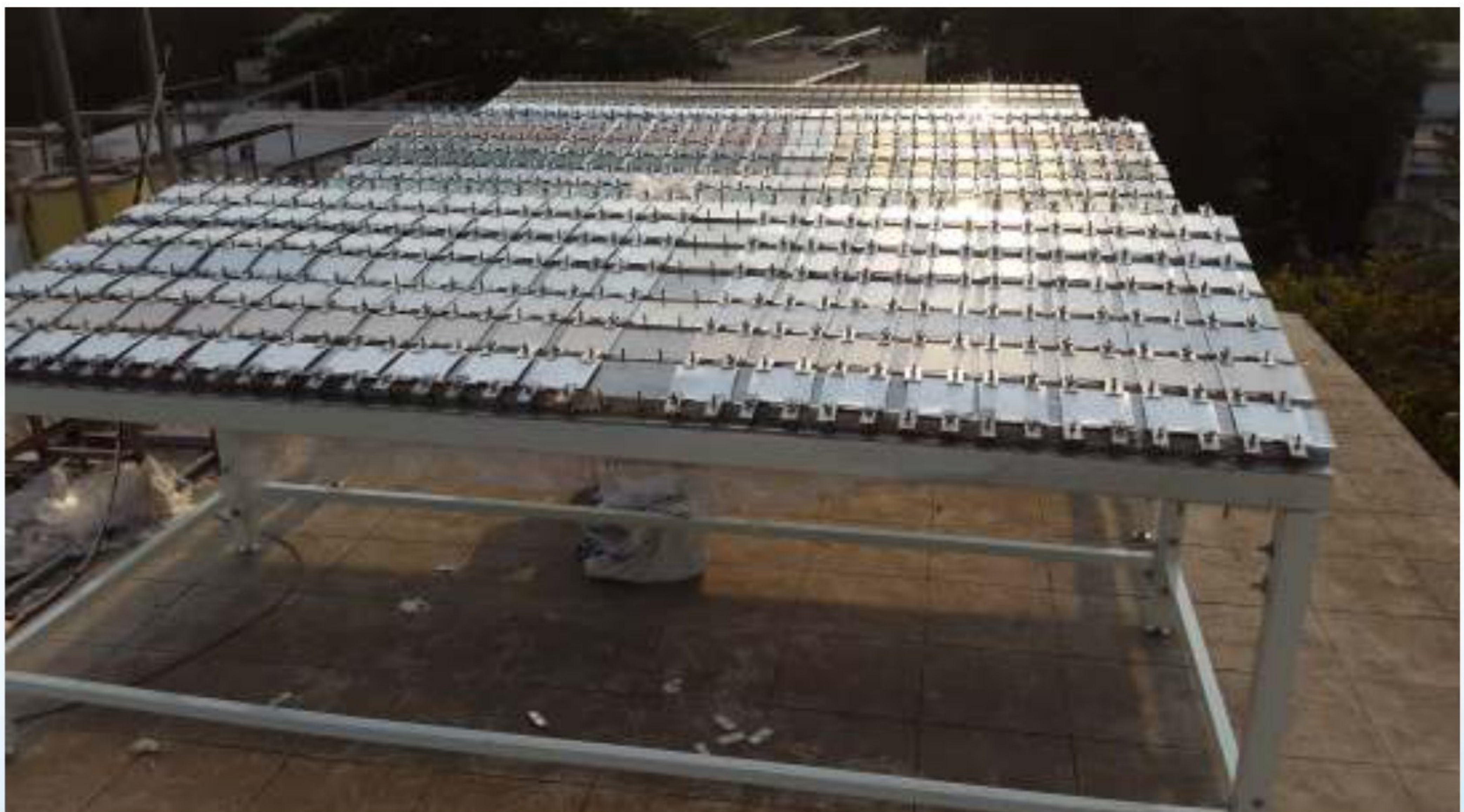
Natural Exposure and Ageing of Cool Roof Specimens- Experiment by International Institute for Information Technology- Hyderabad (IIIT-H) Credit: IIIT-H
